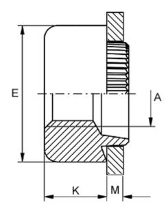
Female thread A = M3Height K = 3.0Outer diameter E = 8.0
